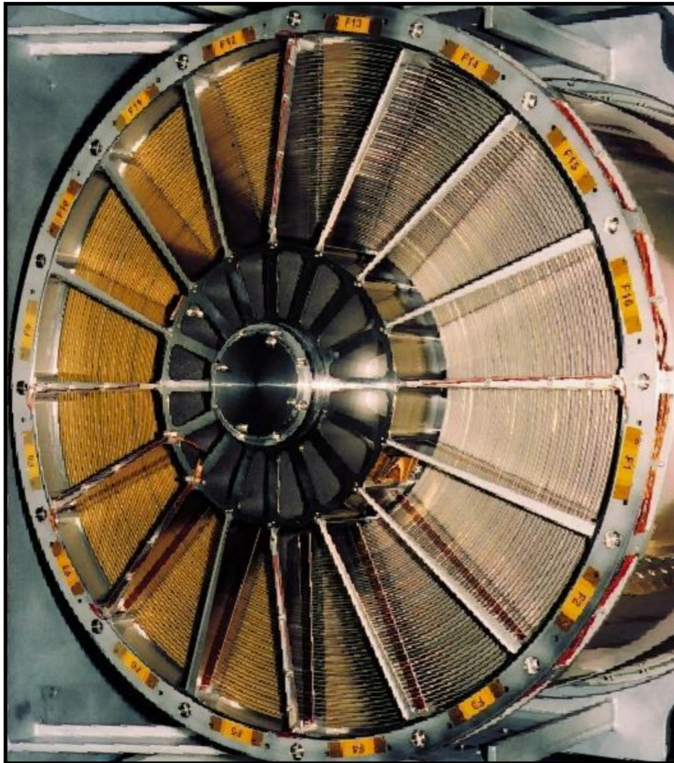
XMM-Newton (0.1–12 keV): 3x58 mirror shells
