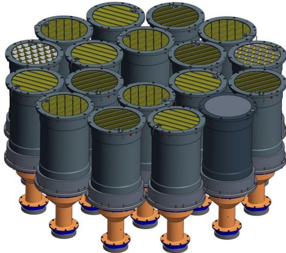
Figure 5 The detector modules and PMTs of Insight -HXMT/HE.
