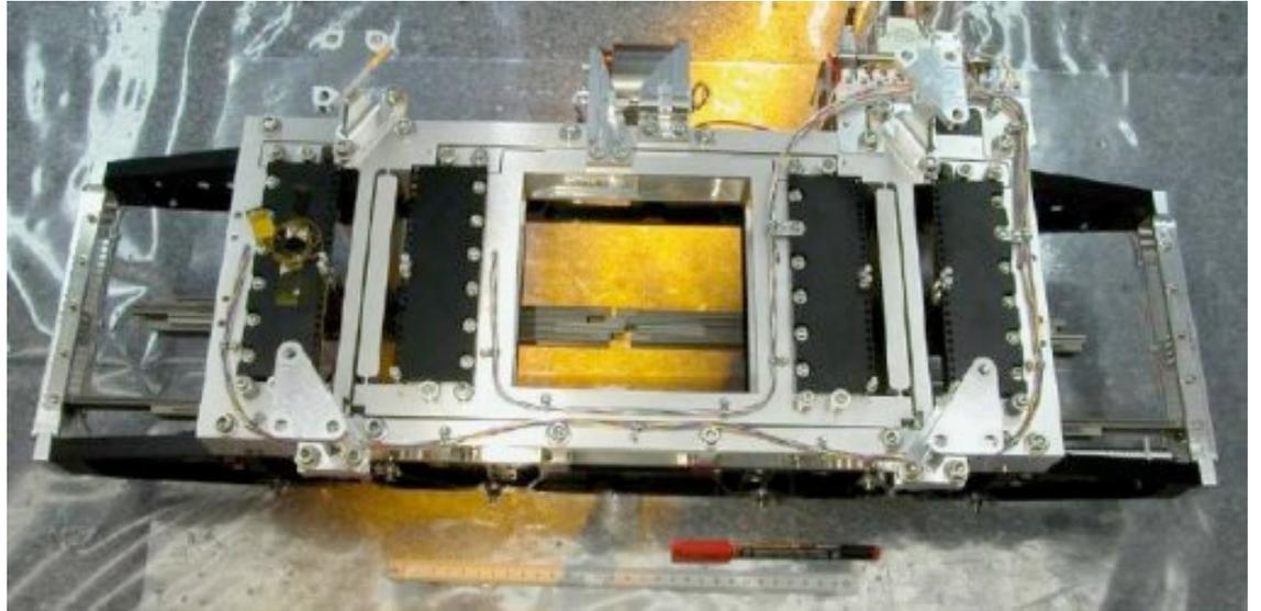
Cryogenic Multi-slit IR spectrograph
